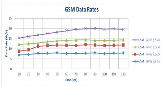
Graph 1: GSM date Rates (CS1, CS2, CS3, CS4)
